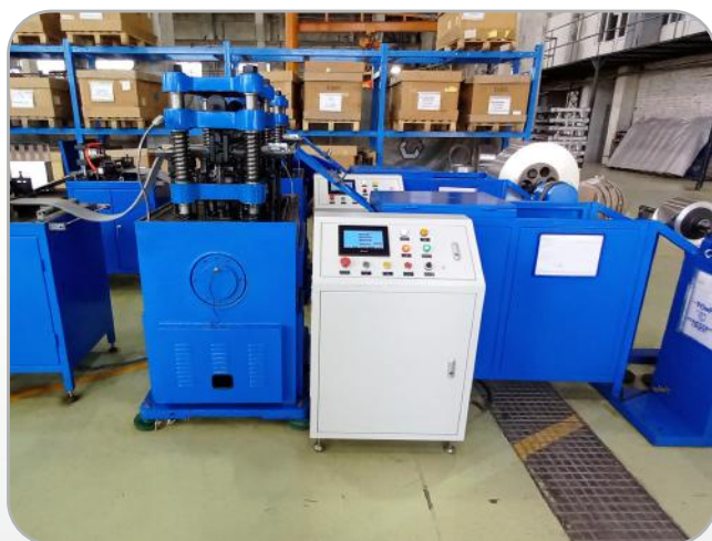
Machine for stamping parts of the skeleton - PARCO (Taiwan)
