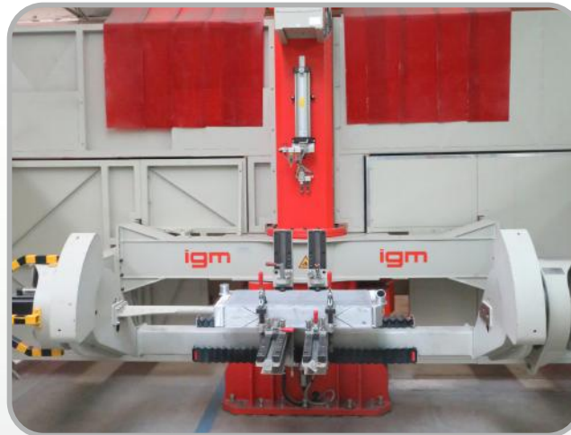
Robotic complex RRMK-602 for arc welding - firm "IGM" (Austria)
