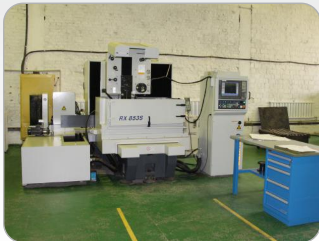
CNC EDM, super drill - CHMER (Taiwan))
