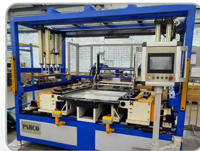
Stand for assembling the core of the heat exchanger - PARCO (Taiwan)
