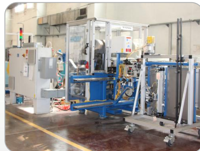
Cooling plate manufacturing line - Voss Manufacturing Inc (USA)
